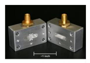
A picture of IBM's "3D" superconducting qubit device where a qubit (about 1mm in length) is suspended in the center of the cavity on a small Sapphire chip. The cavity is formed by closing the two halves, and measurements are done by passing microwave signals to the connectors. Despite the apparent large feature size (the cavity is about 1.5 inches wide) for this single qubit demonstration, the team believes it is possible to scale such a system to hundreds or thousands of qubits.
