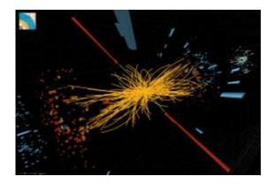
A typical candidate event including two high-energy photons whose energy (depicted by dashed yellow lines and red towers) is measured in the CMS electromagnetic calorimeter. The yellow lines are the measured tracks of other particles produced in the collision. Image: CERN
