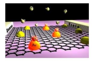
The attachment of hydrogen sulfide gas molecules to the graphene surface results in a drop in current. Credit: A\*STAR
