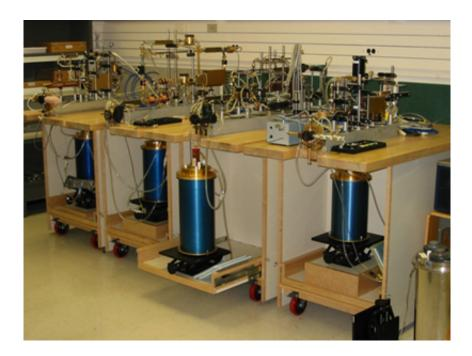
NIST waveguide radiometers. The cryogenic primary standards are encased in the blue cylinders.
