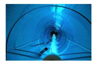
AirUCI researchers simulated smog compounds in the lab by mixing common household chemicals and outdoor air in this 26-foot-long "aerosol flow tube." Credit: Veronique Perraud / AirUCI
