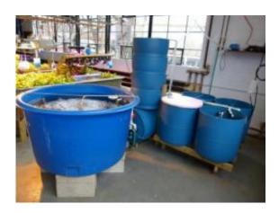
This is a small-scale aquaponics demonstration lab at UMass Amherst. Such recirculating aquaculture systems include various water treatment devices connected through flowing water. The waste stream is diverted to a hydroponic garden (background) where plant roots strip out nutrients. Clean water is then recycled back to the fish holding pens. Credit: UMass Amherst
