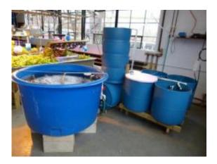
This is a small-scale aquaponics demonstration lab at UMass Amherst. Such recirculating aquaculture systems include various water treatment devices connected through flowing water. The waste stream is diverted to a hydroponic garden (background) where plant roots strip out nutrients. Clean water is then recycled back to the fish holding pens. Credit: UMass Amherst
