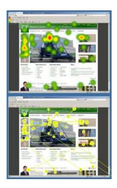
Missouri S&T researchers depict eye-tracking data on a website using a heat map (top image), which shows infrared eye movement, or a gaze plot (bottom image)
