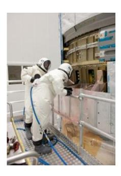
Loading the propellants for ATV Edoardo Amaldi. Since the propellants are hazardous, the operations are performed in 'Scape' suits. In case of a propellant leak, the operators are protected by the suit. Credits: ESA/CNES/Arianespace/Optique Video du CSG-S. Martin
