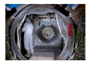
Technicians in Europe's spaceport in Kourou have the delicate task of loading dry cargo into ATV-3 for its journey to the International Space Station in March 2012. Credits: ESA/CNES/Arianespace/Optique Video du CSG-S. Martin 2011
