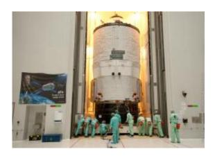
Automated Transfer Vehicle Edoardo Amaldi is moved to the Ariane integration building in Europe's Spaceport in Kourou, French Guiana. From there it will be loaded onto an Ariane 5 rocket for launch in March 2012. ESA's third automated space freighter will carry about two tonnes of dry cargo, 285 kg of water and more than three tonnes of propellants to the International Space Station. Credits: ESA/CNES/Arianespace/Optique Video du CSG - P.Baudon
