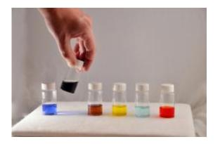
Sandia researchers have discovered a new family of liquid salt electrolytes that could lead to batteries with three times greater energy density than other available storage technologies. The MetILs are, from left to right: copper-based compound, cobalt-based compound, manganese-based compound, iron-based compound, nickel-based compound, and vanadium-based compound. (Photo by Randy Montoya)
