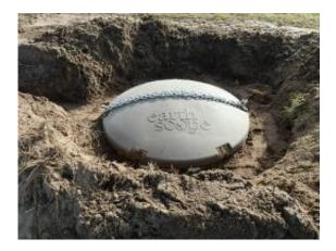
A vault with the transmitting seismometer is closed, then a mound of dirt is piled on top.Credit: IRIS
