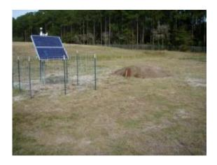
Transportable Array Station 457A in Florida: first such seismic station on the U.S. East Coast. Credit: IRIS
