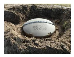
A vault with the transmitting seismometer is closed, then a mound of dirt is piled on top.Credit: IRIS
