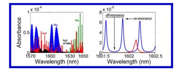
Absorption of photons at different wavelengths from 1.57 to 16.5 micrometers for water and each of the principal greenhouse gases. Right: Difference in absorption by carbon dioxide of photons on- and off-resonance.
