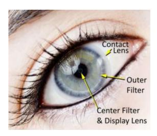
Currently being developed by DARPA researchers at Washington-based Innovega iOptiks are contact lenses that enhance normal vision by allowing a wearer to view virtual and augmented reality images without the need for bulky apparatus.
