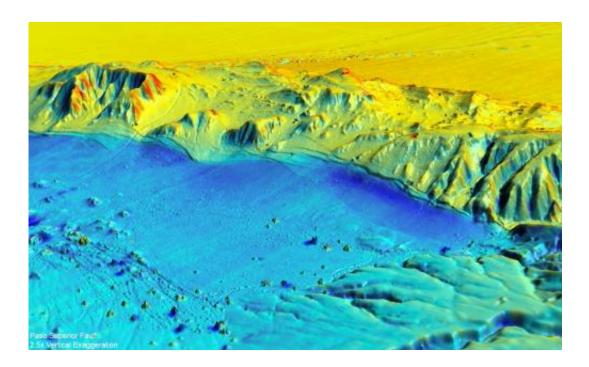
This is a visualization of LiDAR data from the April, 2010 earthquake near Mexicali. Blue shows where ground surface moved down, red shows upward movement compared to the previous survey. Credit: Michael Oskin, UC Davis
