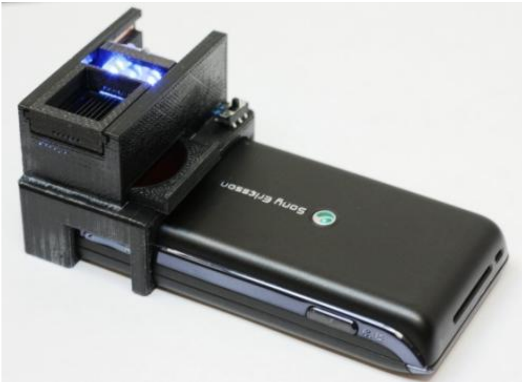
Cell phone-based E. coli detector. Image courtesy of UCLA Engineering
