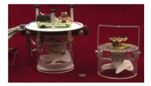
The LED-based insect trap (right) is smaller and lighter and uses less energy than traditional light-based collection devices.
