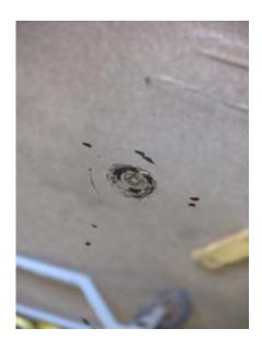
Cracks in the secondary mirror on the Blanco telescope in Chile after an accident on February 20, 2012. Credit: Cerro Tololo Inter-American Observatory
