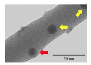
Scanning transmission electron microscope image of a polystyrene nanowire containing iron oxide nanoparticles. The yellow arrow shows the surface of the nanowire, and the red arrow shows iron oxide nanoparticles which exist in the interior of the nanowire. (Photo courtesy of Hitachi High-Technologies Corporation)
