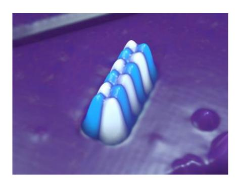
welve iron atoms make up the world's smallest magnetic data storage unit to date. The antiferromagnetic order in the iron atom array is revealed by spin-polarized imaging with a scanning tunneling microscope. Credit: Sebastian Loth/CFEL
