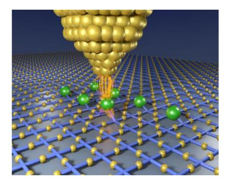
This graphic shows the atomically precise assembly of an atomic-scale antiferromagnet with the tip of a scanning tunneling microscope. Iron atoms are placed onto a copper nitride surface and bound by two nitrogen atoms (blue rods) into a regular array separated by one copper atom (yellow). Credit: Sebastian Loth/CFEL
