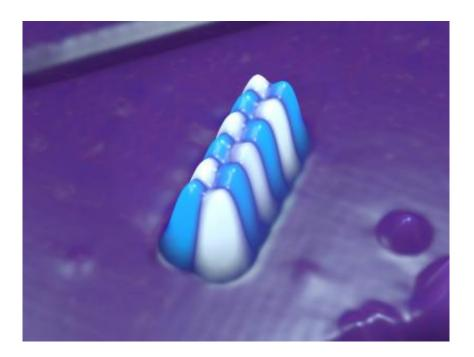
welve iron atoms make up the world's smallest magnetic data storage unit to date. The antiferromagnetic order in the iron atom array is revealed by spin-polarized imaging with a scanning tunneling microscope. Credit: Sebastian Loth/CFEL
