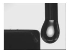
The effect of a hand held magnet on a drop of surfactant solution.
