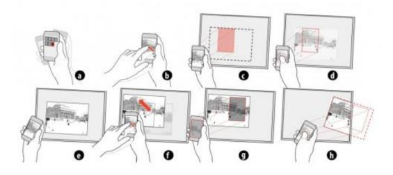
Virtual Projection walkthrough: (a) Shaking the device to create a view. (b) Interacting with a non-projected view. (c-e) Creating a projection by aiming at the secondary display, long pressing, and releasing. (f) Synchronized interaction. (g) Projection frustum can be used for filtering or navigating. (h) Projections can be moved or deleted by aiming, long pressing, and dragging out of the display. Image credit: Dominikus Baur, et al. Proceedings of CHI 2012 (preprint)
