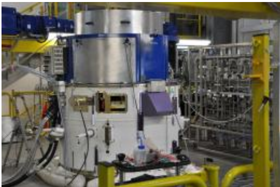
Vega's AVUM - Attitude & Vernier Upper Module - liquid-propellant fourth stage. Credits: ESA
