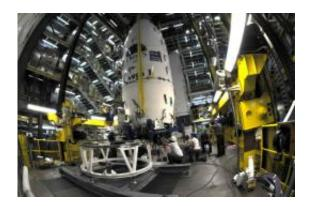
Vega's upper composite, comprising LARES, ALMASat-1, seven CubeSats and the fairing, was transferred to the pad on 24 January and added to the vehicle at Europe's Spaceport in French Guiana. Credits: ESA - M. Pedoussaut, 2012
