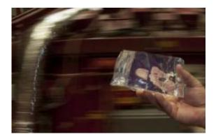
Twenty-one tons of borosilicate glass chunks, melted at a temperature of 1,170 degrees Celsius (2,140 F), went into making the second mirror for the GMT. (Photo: Patrick McArdle/UANews)
