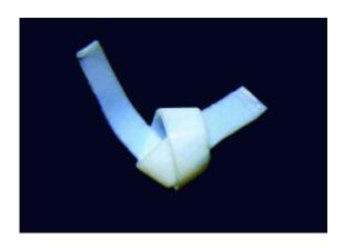
(PhysOrg.com) -- Delicate and translucent as a puff of air, yet mechanically stable, flexible, and possessing amazing heat-insulation properties—these are the properties of a new aerogel made of cellulose and silica gel. Researchers led by Jie Cai have introduced this novel material, which consists almost completely of air, in the journal *Angewandte Chemie*.
