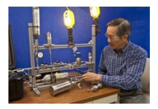
Dr. Kit Heung of Savannah River National Laboratory demonstrates a system incorporating a fuel cell and light-weight hydrogen storage material. SRNL's advances in the use of alane, a lightweight material for storing hydrogen, are paving the way for the successful development of portable power systems with capacities that far exceed the best batteries available today. Credit: Savannah River National Laboratory
