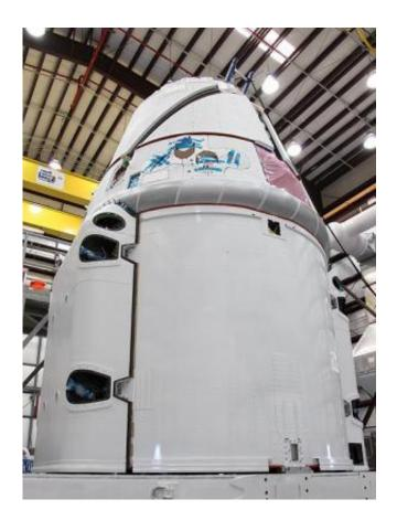
This SpaceX Dragon will launch to the ISS sometime in 2012 on COTS2/3 mission. Protective fairings are installed over folded solar arrays, at the SpaceX Cape Canaveral launch site.
