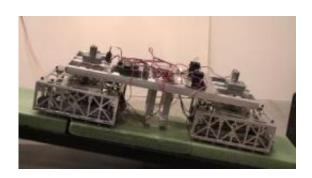
Scalybot 2, built by Georgia Tech, is designed to be a a more efficient searchand-rescue robot. It was designed based on the movements of snakes. Credit: The Georgia Institute of Technology
