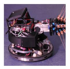
The Shrewbot, which is the latest in a series of robots to use 'active touch' rather than vision to navigate their environment.
