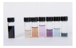
Armchair-enriched batches of nanotubes show their colors in an array of varying types. The vial at left is a mix of nanotubes straight from the furnace, suspended in liquid. The vials at right show nanotubes after separation through ultracentrifugation. Excitons absorb light in particular frequencies that depend on the diameter of the tube; the mix of colors not absorbed are what the eye sees. (Credit: Erik Hároz/Rice University)
