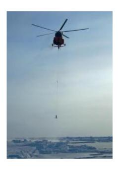
An instrument about to be dropped through an opening in the ice to the seafloor will record ocean bottom pressure to compare with similar data recorded by NASA's GRACE satellites. Data from GRACE, ICESat and actual water samples led to the discovery of a new pathway of freshwater in the Arctic. Credit: C. Peralta-Ferriz/UW Applied Physics Laboratory
