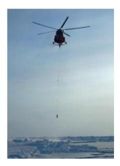
An instrument about to be dropped through an opening in the ice to the seafloor will record ocean bottom pressure to compare with similar data recorded by NASA's GRACE satellites. Data from GRACE, ICESat and actual water samples led to the discovery of a new pathway of freshwater in the Arctic. Credit: C. Peralta-Ferriz/UW Applied Physics Laboratory
