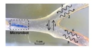
Researchers in South Korea demonstrated a microrobot moving through a structure intended to simulate the environment of a blood vessel. The microbot can move up and down (1 and 2), and wiggle through the simulated vessel in a helical motion (2, 3, 5, 6). Credit: S.M. Jeon, Hanyang University, et al
