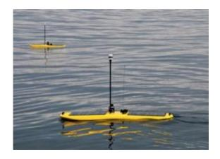
Wave Gliders can be released off the coast and operate along survey lines running perpendicular to the coast.
