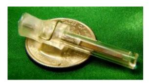
Researchers have created a new type of miniature pressure sensor, shown here, designed to be implanted in the body. Acoustic waves from music or plain tones drive a vibrating device called a cantilever, generating a charge to power the
