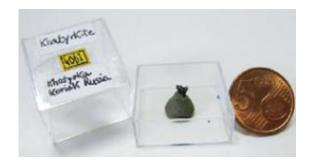
The researchers studied a small sample of the mineral khatyrkite, which is mounted on a pyramid-shaped piece of clay next to a penny to illustrate the small size of the sample. Credit: Paul Steinhardt
