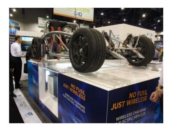
(PhysOrg.com) -- Qualcomm has demonstrated its new wireless power transmission system for electric vehicles (EVs) at the Consumer Electronics Show (CES). The system, including one pad for power transmitting, another for power-receiving, and control unit, uses the inductive transfer method to charge an EV. The chip-maker's
