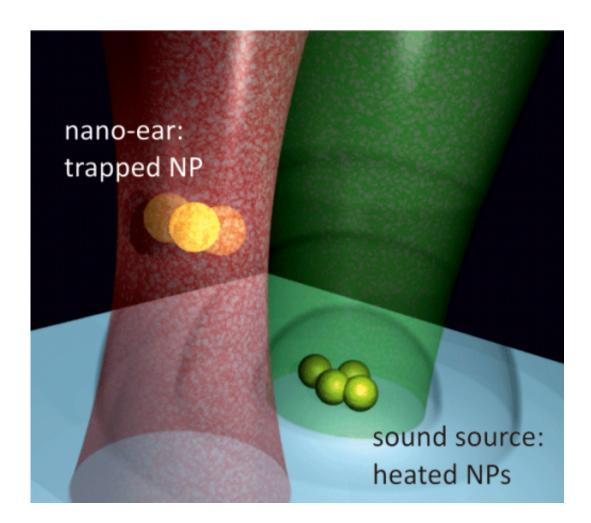
An optically trapped nanoparticle can act as an ultrasensitive detector of sound. Pressure waves from a nearby sound source are detected by tracking the small displacements of a trapped gold nanoparticle from its equilibrium position in the neck of a focused laser beam (red region). The sound waves are produced by an aggregate of nanoparticles that vibrate when heated by a laser (green region). Image: A. Ohlinger et al., Phys. Rev. Lett. (2012)
