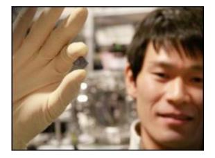
Koji Usami shows the holder with the semiconductor nanomembrane. The holder measures about one cm for each link, while the nanomembrane itself has a surface area of 1 times 1 millimeter and a thickness of 160 nanometers. Credit: Niels Bohr Institute
