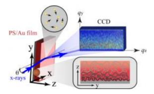
Schematic configuration of the marker XPCS experiments. The use of resonance enhanced X-ray scattering for XPCS enables one to intensify, by more than one order of magnitude, the probing electrical field in the regions of interest within single nanometer polymer films.
