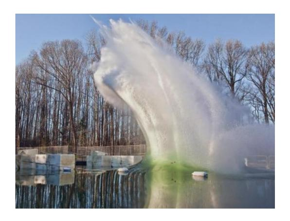
The Jan. 06, 2012, Orion test article water landing drop test.
