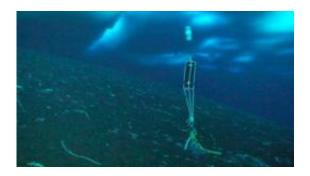
The image shows a SeaFET pH sensor deployed underneath approximately 12 feet of sea ice in McMurdo Sound, Ross Island, Antarctica, in Oct. 2010. Scientists use these sensors to identify the natural dynamics of ocean pH in order to better understand how marine organisms may be impacted by climate change. The black object is the sensor, which is anchored to the ocean bottom using weights. Along the ocean bottom, worms and sea stars are visible. Credit: Rob Robbins
