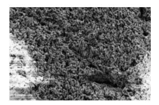
Electron microscope image of the microbe, Geobacter sulfurreducens, the core of the microbial fuel cell-based system.
