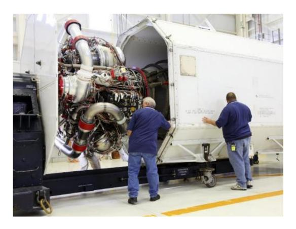
Technicians oversee the installation of a Pratt Whitney Rocketdyne RS-25D engine into a transportation canister in the Engine Processing Facility at Kennedy Space Center, Fla. The 15 engines used during the Space Shuttle Program will moved to Stennis Space Center in south Mississippi, where they will be stored for future use on NASA's new deep space heavy-lift rocket, the Space Launch System. Credit: NASA/KSC
