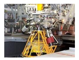
The J-2X powerpack assembly is successfully installed and ready for testing of the turbomachinery components. Credit: NASA/SSC
