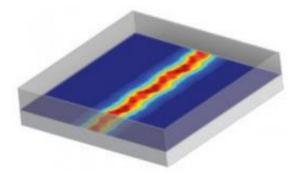
Wires just one atom tall have been created by inserting a string of phosphorus
