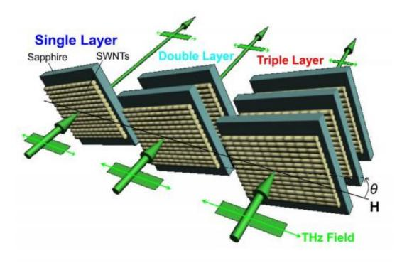
A triple layer of carbon nanotube arrays on a sapphire base are the basis for a new type of terahertz polarizer invented at Rice University. The polarizer could lead to new security and communication devices, sensors and non-invasive medical imaging systems. (Credit: Lei Ren/Rice University)
