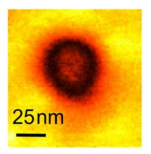
ORNL researchers used piezoresponse force microscopy to demonstrate the first evidence of metallic conductivity in ferroelectric nanodomains. A representative nanodomain is shown in the PFM image.
