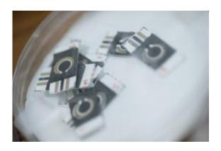
Biosensor chips for use in handheld devices for detecting biohazards in the field, developed by biosystems and agricultural engineering professor Evangelyn Alocilja. Credit: Kurt Stepnitz
