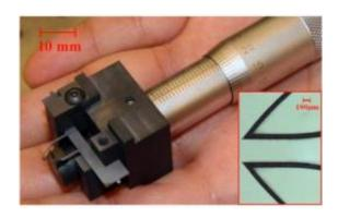
Purdue researchers have created a new type of microtweezers capable of manipulating objects to build tiny structures, print coatings to make advanced sensors, and grab and position live stem cell spheres for research. Credit: Birck Nanotechnology Center
