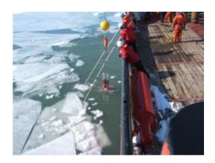
Environment Canada and Canadian Coast Guard personnel recover a sediment trap from an icebreaker on an ice-covered Lake Erie in February 2010. Sediment traps are placed on the bottom of a lake to measure the how much algae sink to the bottom. In this case, algae are thriving in winter below ice. Credit: Michael Twiss, Clarkson University)
